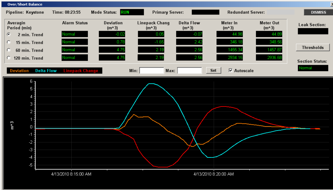
Figure 2: Simulator depiction of pipe section balancing trend during for a pump start up.
