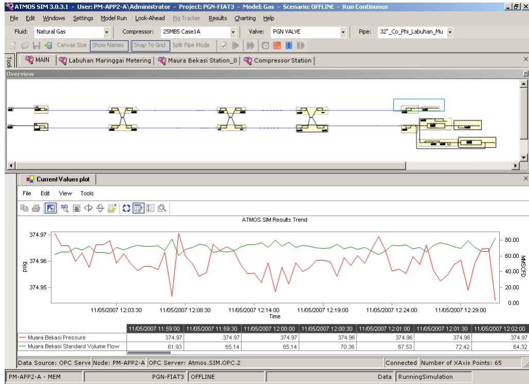
Figure 5 – The Network Model of the PGN Pipeline and the Flow/Pressure Trend at a Delivery Point
